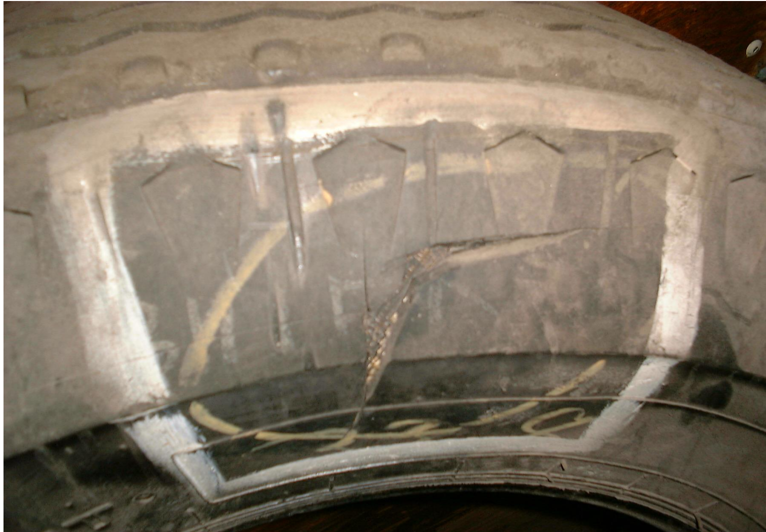
Tire sidewall cut/punctured, exposing belt material – J2 Condition
