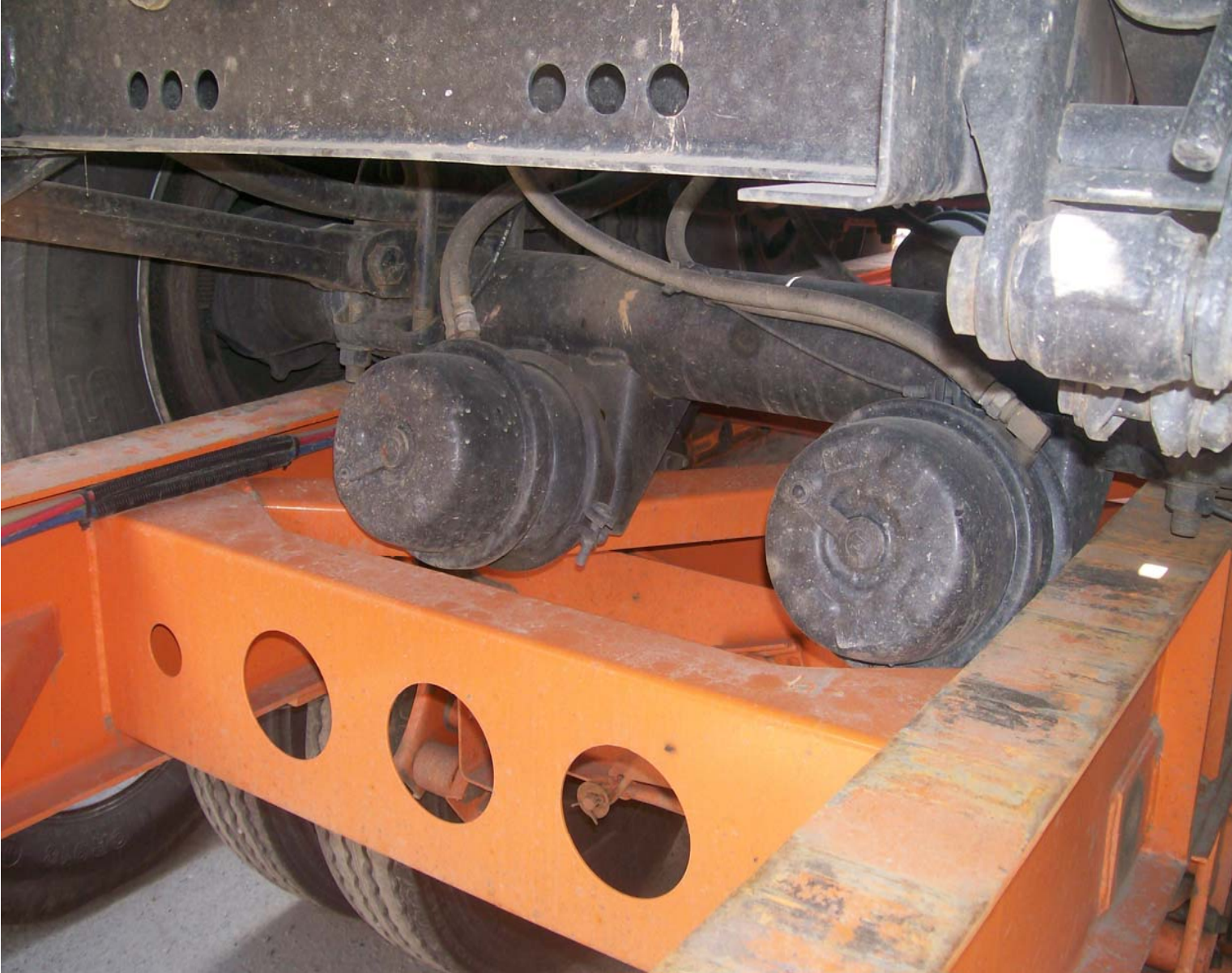
Brake Chamber damage caused by improper chassis stacking
